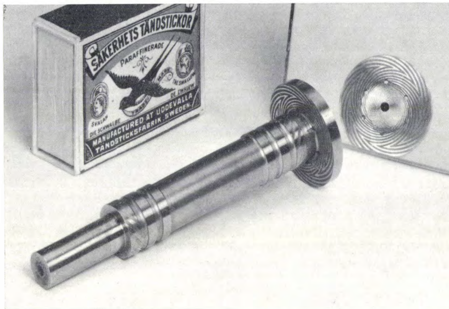
Fig. 6. The fixed shaft with thrust bearing (flange which has a spiral-groove pattern on both sides) and two journal bearings, each consisting of two sections. Helical grooves on the left and right keep the lubricant in the bearings at the correct pressure.
