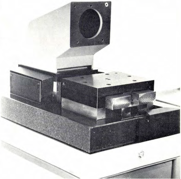
Fig. 9. The slide systems of a six-barrel step-and-repeat camera. The carriage on which the photographic plates are mounted can be seen at the front, and the carriage at the back carries the projection systems on an arm, here already fitted.
