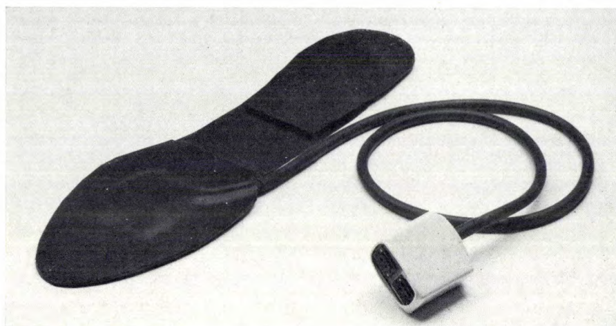
Fig. 2. Insole with flexible tube and pneumatic switch.
