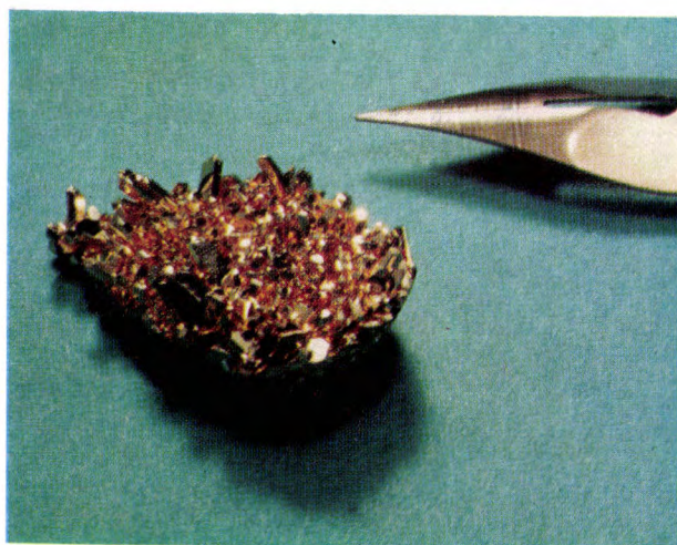
Fig. 10. Group of gold crystals of about 10 grammes, obtained by heating gold (without temperature gradient) in 10-molar \text{HI} for 10 days at 500^\circ\text{C} . The title photograph shows gold crystals grown in a temperature interval of 480 \rightarrow 500^\circ\text{C} .
