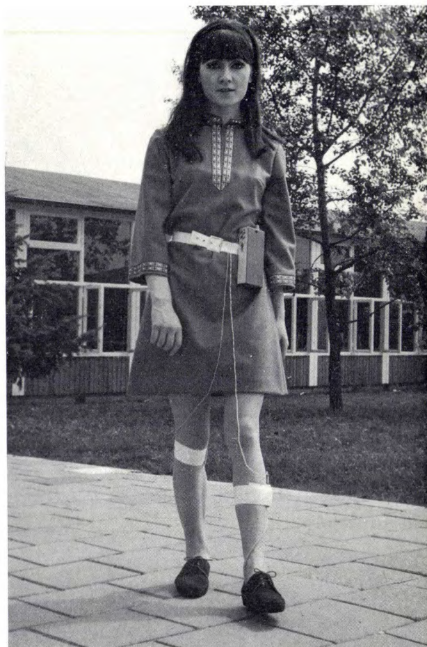
Fig. 1. The muscle stimulator in use. A rubber insole containing a small air chamber, connected by a flexible tube to a pneumatic switch, is fitted in the shoe on the unaffected foot. When the patient walks, the pneumatic switch (attached to the lower leg by means of an elastic bandage) is operated and switches the stimulator on and off. The stimulator, which is carried on a belt around the waist, applies pulses to an electrode in the elastic bandage around the affected leg.
